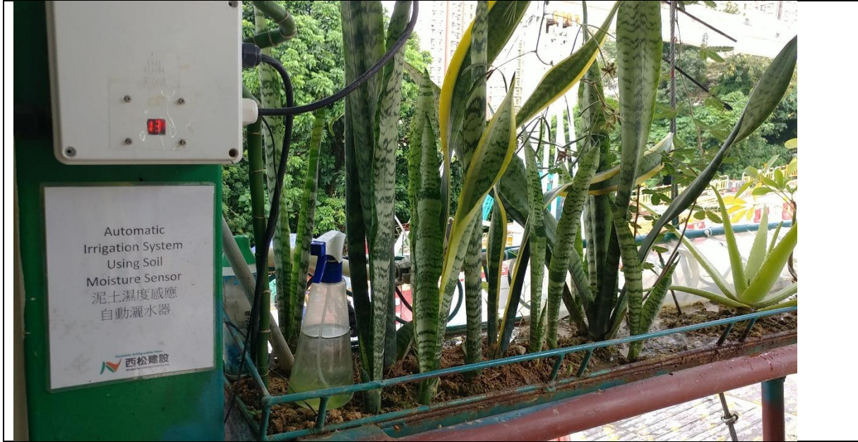
Automatic irrigation system using soil moisture sensor is used for irrigation of plant.
